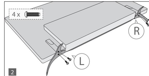
1. (fig.1) Place the TV set on a flat and clean surface with the panel facing downwards to avoid damage. (fig.2) Secure the stand feet to the underside of the TV set using the 4 screws provided. The stand feet are marked L (left) and R (right).
